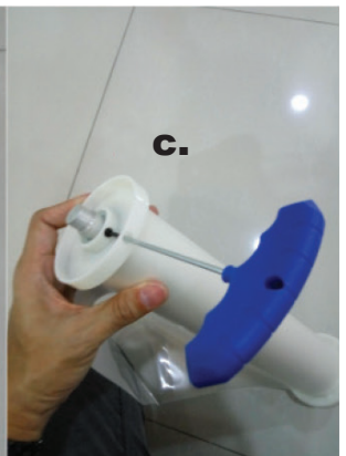
4. Load the roll of film onto the film mandrel. (same process for top and bottom mandrels). a. Unlock the left side, slide roll of film onto mandrel b. Line up the slot lines, place end cap back on mandrel c. Tighten the screw with tool provided
