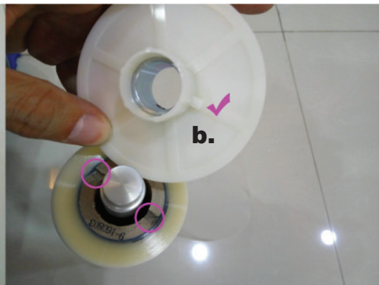
4. Load the roll of film onto the film mandrel. (same process for top and bottom mandrels). a. Unlock the left side, slide roll of film onto mandrel b. Line up the slot lines, place end cap back on mandrel c. Tighten the screw with tool provided
