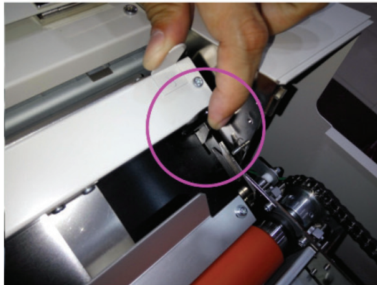
3. Press the left and right brackets and lift the front direction board feeder up gently.
